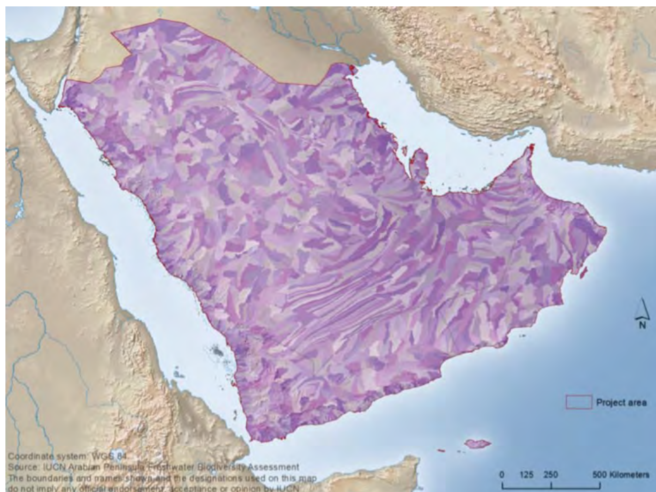
Fig. 2.1 River subcatchments as delineated by HydroSHEDS used to map and analyse species distributions.
