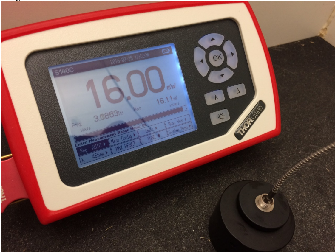
Image 3 shows the light testing equipment in action, each implant passed the minimum requirement of 5 mWs of 465 nm light wavelength emission.
