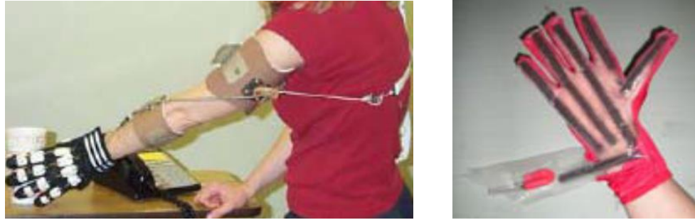
FIGURE 12. BODY-POWERED ORTHOSIS (LEFT) AND PNEUMATIC-POWERED DEVICE (PPD) (FROM LUO ET AL., 2005).
