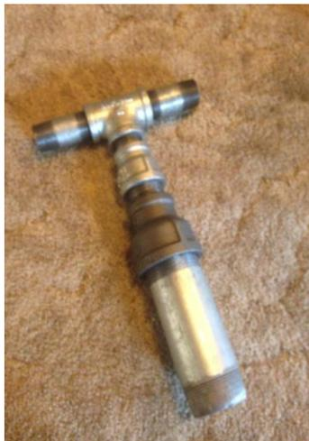
**Figure 2** Soil Sampling Tool
