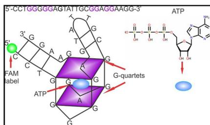
Figure 2: ATP aptamer sequence (top left) and a schematic of the folding of the aptamer sequence into a secondary structure consisting a stem, hairpin, G-quartets and a binding pocket for small molecule ligands (blue oval representing ATP ligand). The structure of ATP is shown on the top right. The aptamer sequence was labeled with 6-carboxyfluorescein (FAM) (green solid circle) for fluorescence detection.
