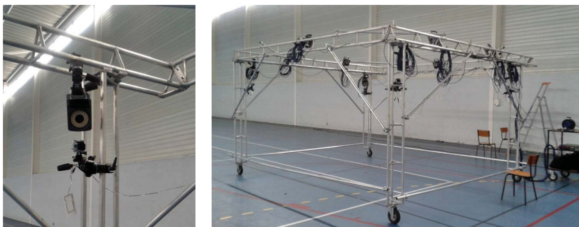
Figure 1. Cameras position (ViconMX40 and GoPro, Hero3 +) fixed in a rigid structure that moves.
