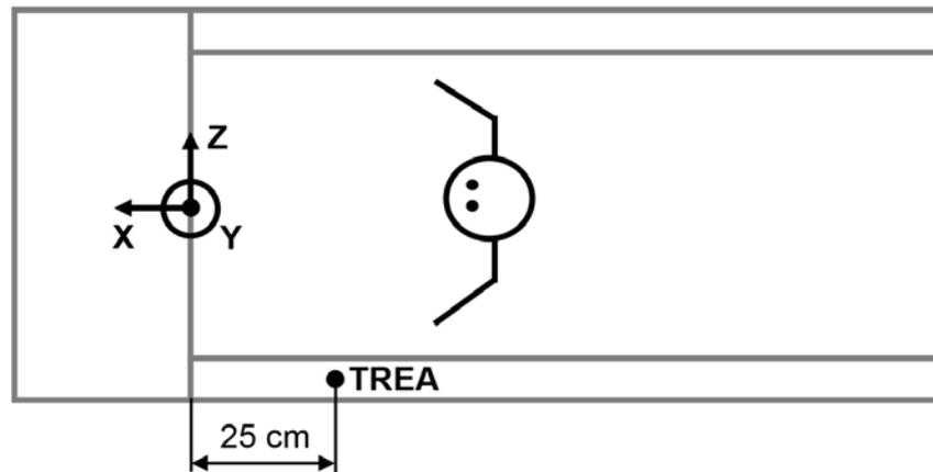
Figure 1: Treadmill with TREA marker and global coordinate system.
