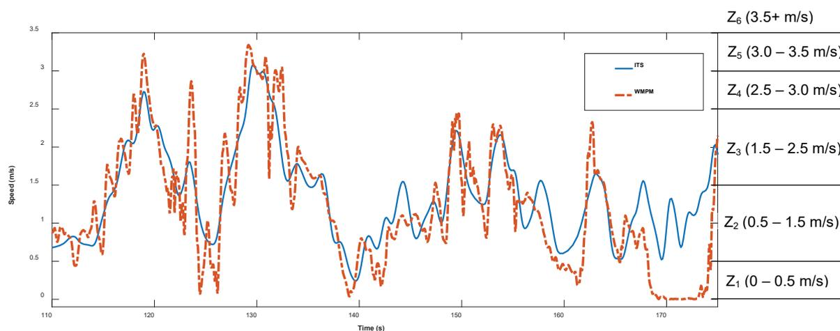
**Figure 2: Typical example of the speed signal by the ITS and WMPM, showing small differences in speed pattern e.g. while pushing (112-119s) and turning on the spot (168-174s).**
