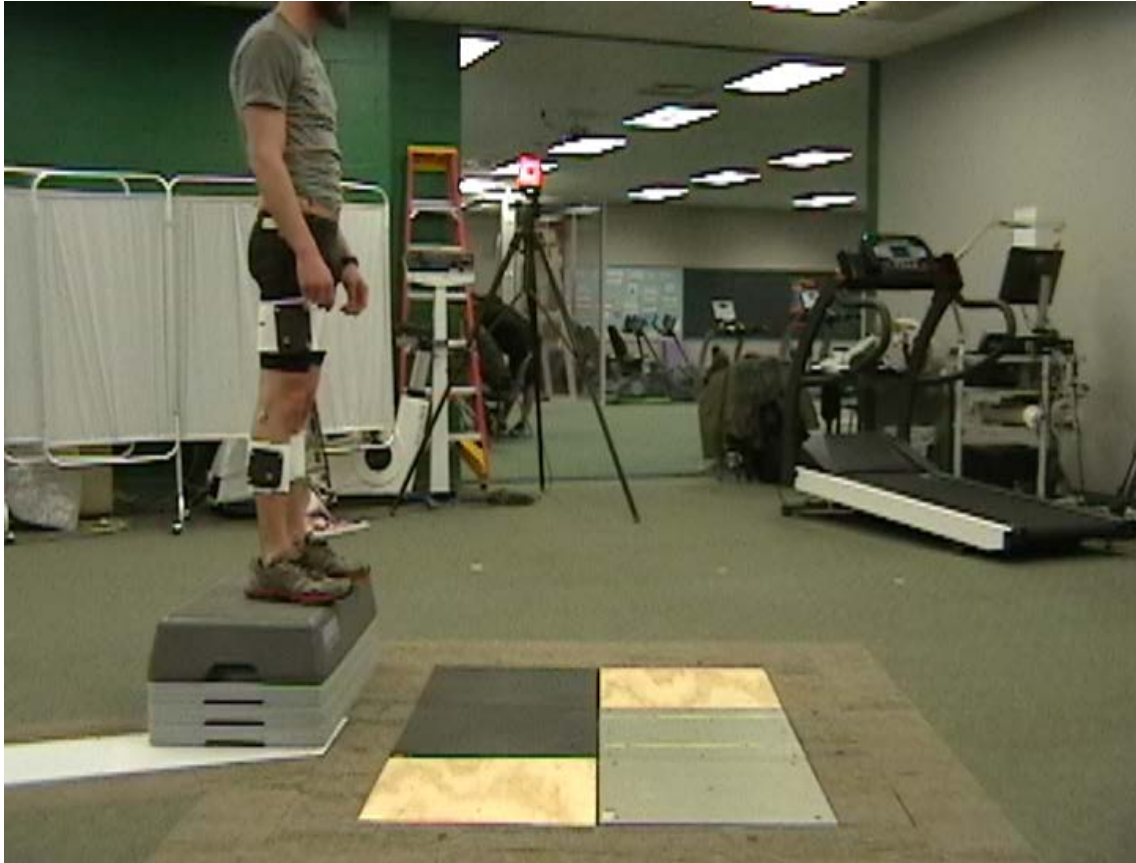
FIGURE 3. To perform the drop vertical jump test, subjects started from this 31 cm tall box and landed with one foot on each of the force plates below, then immediately performed a maximal jump.
