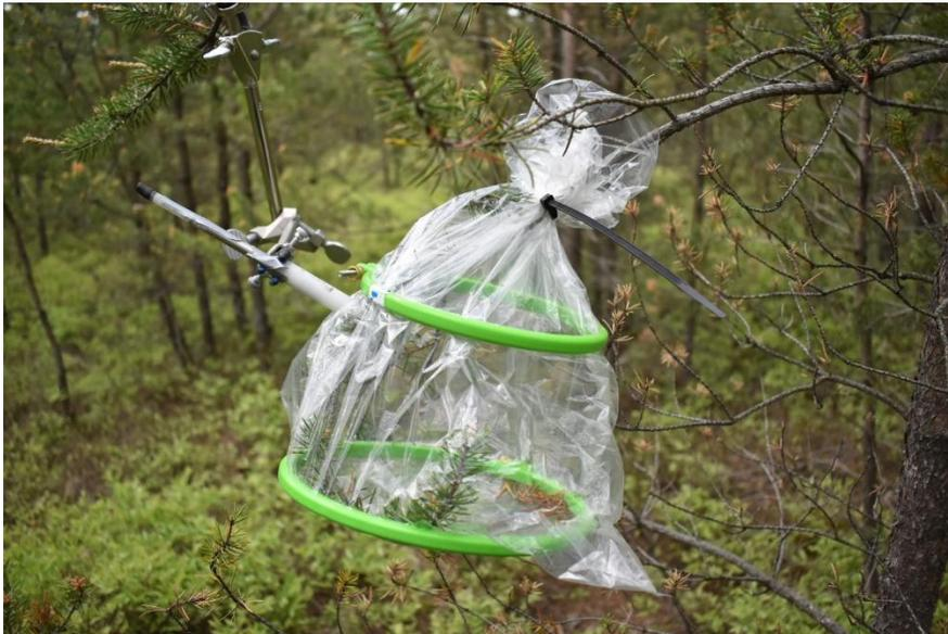
**Fig 2** Stable headspace for VOC sampling using an oven bag (Reynolds, slow cooker liners 13inx21in), two embroidery hoops (one 8 inches in diameter and a second 6 inches) for stability, and zip-ties to fasten gently to the tree. Fiber holder is held by
