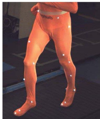
Figure 2: Body suit and reflective markers.
