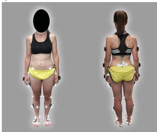
Figure 1 Subject with attached markers and IMUs.
