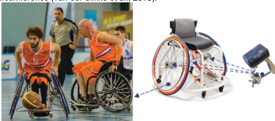
Figure 1: Measurement setup, with IMUs on wheels and frame applied during match measurements. (Photograph by www.frankvanhollebeke.be ).
