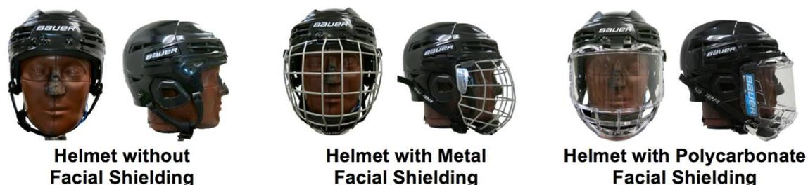
**Figure 1: Anterior and lateral views of the helmet/facial shield conditions fitted on a medium sized NOCSAE headform.**
