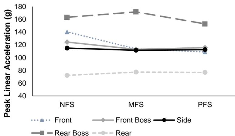
**Figure 2: Impact locations and facial shielding conditions. Note that the facial shielding conditions on the horizontal axis are represented by grouping labels: no facial shielding (NFS), metal facial shielding (MFS), and polycarbonate facial shielding (PFS). Impact locations are represented by different lines.**
