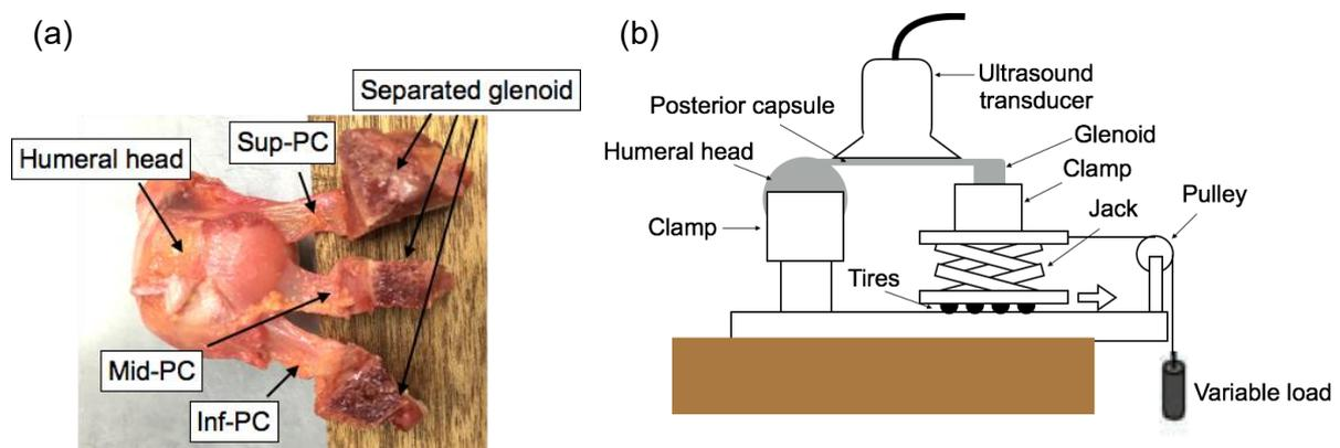
**Figure 1: (a) Posterior capsules specimens of the right shoulder. (b) Experimental setup. The humeral head and the glenoid were fixed. Passive force for the capsules was applied to the glenoid through a pulley system.**
