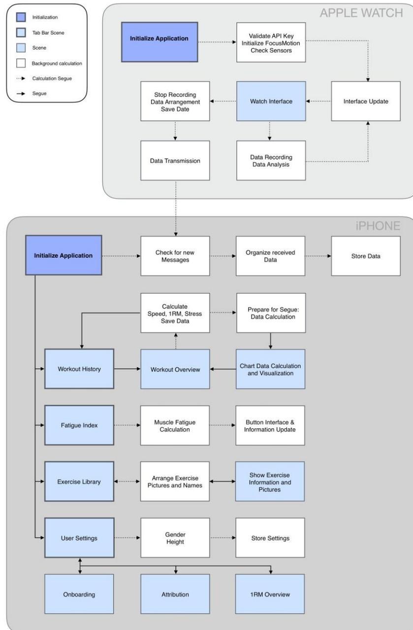
**Figure 1: Workflow of the watchOS and iOS application running process presenting all programmed scenes, segues and calculations.**
