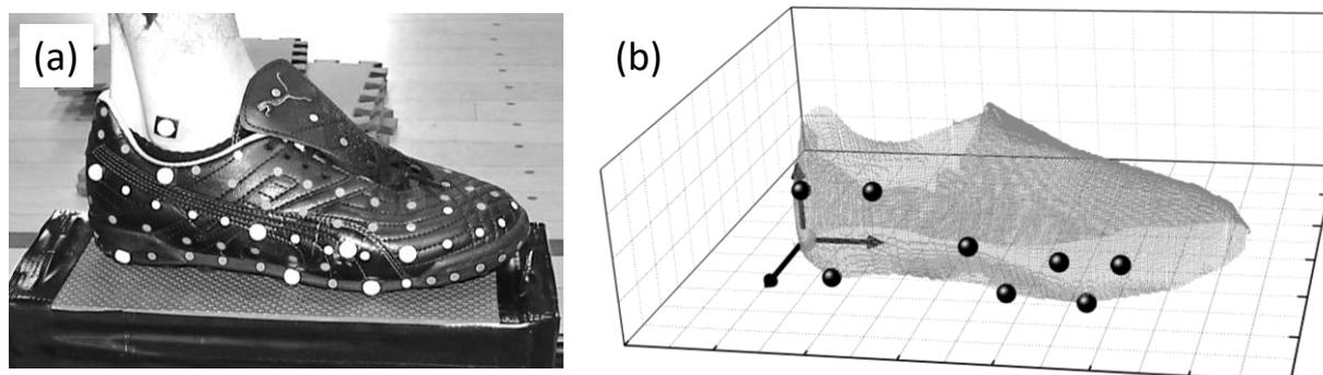
**Figure 1. (a) The shoe for the standing calibration. The white markers are criteria markers. (b) The foot shape which represented by the dots along the shoe surface.**
