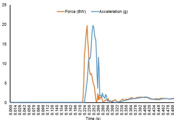
**Figure 3: Example force and acceleration-time curves from the force platform and IMU measuring tools. Note that the two measuring tools were not time synchronised.**
