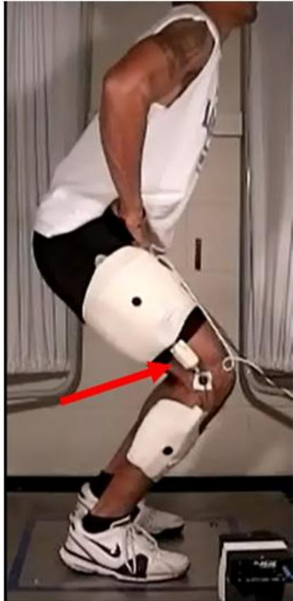
**Fig. 1** Markers (black dots) and El-Gon (arrow) placement.
