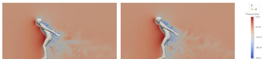
**Figure 7: Pressure distribution in the sagittal plane of the jumper at 0.5 s**
