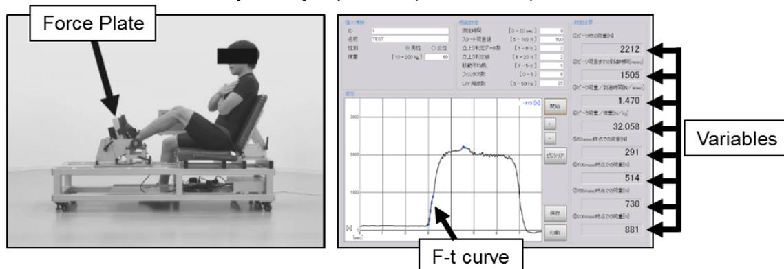
Figure 1 Measuring equipment: the multi strength tester and posture of a participant during measurement (left) and the display that shows the measurement results (right)
