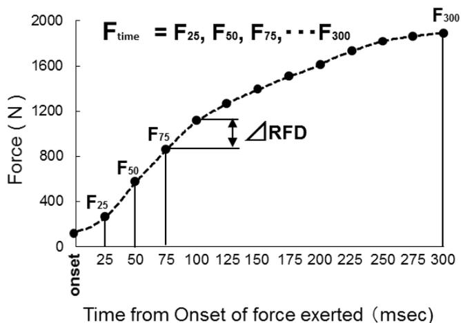
**Figure 2: Calculation of the RFDs during leg extension.  $F_{\text{time}}$ : The force at the specific time points (defined as  $F_{25}$ ,  $F_{50}$ ,  $F_{75}$ , etc.).  $\Delta\text{RFD}$ : The force development in 25 ms (0-25, 25-50, ... 275-300).**
