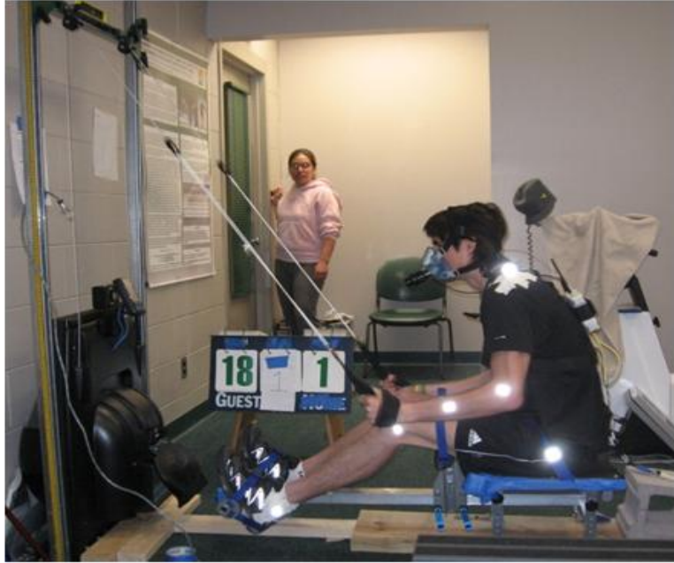
Figure 2. The modified VASA Ergometer, during a Seated test.
