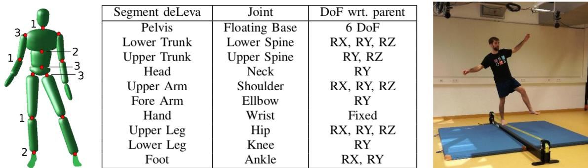
**Figure 1: Left: Overview of the degrees of freedom (DoF) used for the deLeva Model. The Floating Base is not actuated and has three rotational and three translational DoF. The actuated rotational joints of the model are indicated with R and X, Y and Z describe the according coordinate system axis. Right: A typical slackline situation in the motion capture lab. The slackline is 5cm wide and 3m long and installed with the Gibbon Slackrack 300.**
