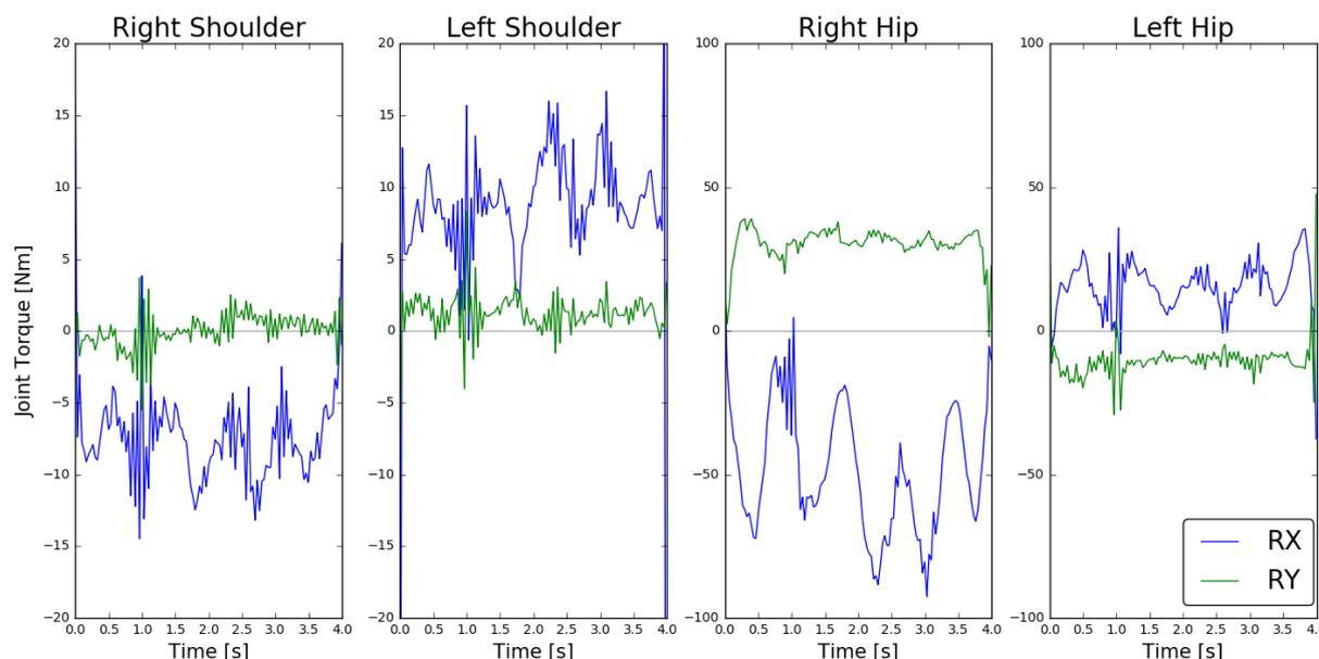
**Figure 2: The resulting joint torques of the model for hip and shoulders joints. Higher actuation is seen in the coronal plane (RX) than for the sagittal plane (RY). Balance in ML direction is maintained by using the arms and legs, while the AP is balanced with the supporting leg's hip joint.**
