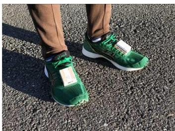
Figure 1: IMU sensors on shoes
