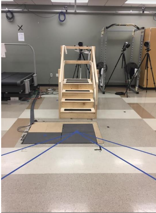
Figure 2: Protocol set-up, frontal and overhead view: Staircase, force platform and colored-tape trail.
