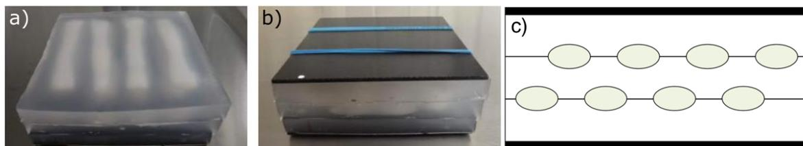
**Figure 2: Eight tendons: a) alternately layered between water like gel pads; b) stabilized through thin plastic plates and rubber bands; c) cross section sketch of phantom.**
