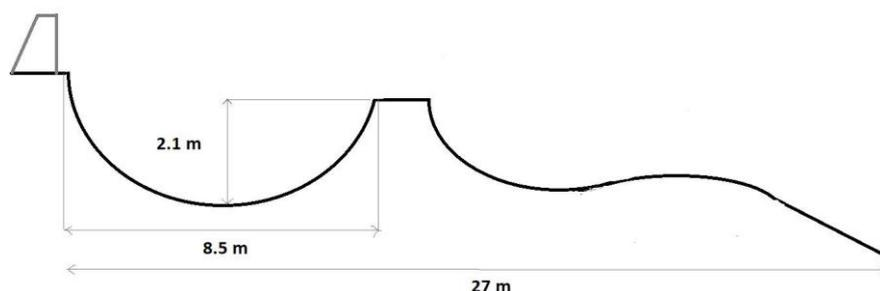
**Figure 1: Dimensions of the start area.** (Drawing is not to scale; the start platform was about 0.4 m higher than the highest point of the Wu-Tang).
