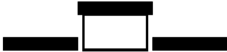
Figure 2. Schematic of lateral view of stepping apparatus, containing 3 AMTI force platforms. Height of the middle step was 18 cm. Area of the step was 0.23 m 2 .
