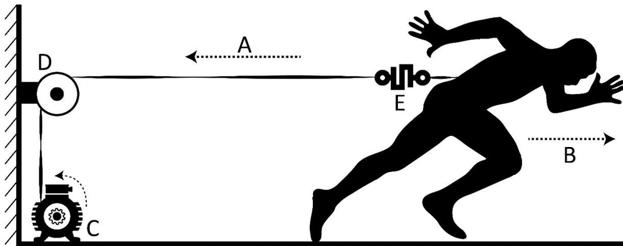
**Figure 1: Conceptual drawing of the winch towing system. A=The direction the athlete moves due to the winding in of the motor, B=The direction of the force the athlete produces and tries to resist the motion, C=The motor winding in the tether/cable, D=A pulley that guides the tether/cable, E=S-beam load cell.**
