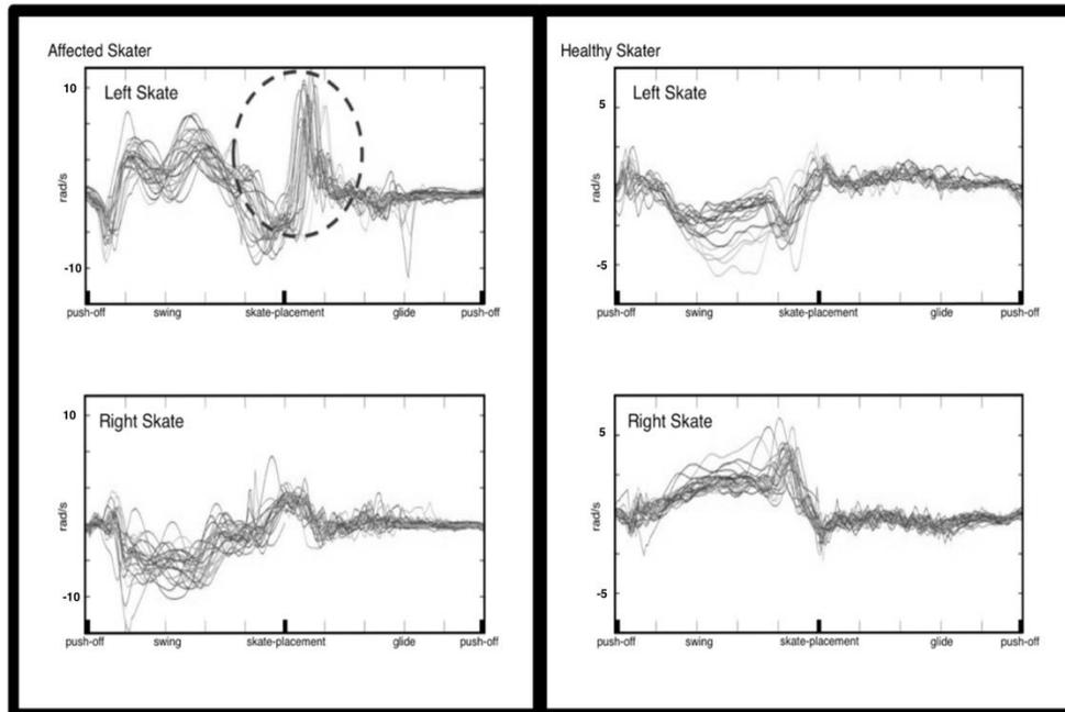
**Figure 2:** Participant one, angular velocity (rad/s) around the vertical (z axis) for 30 normalized gait cycles are portrayed for an affected and healthy skater. The dystonic skater's cramp (circled) occurs always either directly before, or directly after skate placement. The aberrative jerking motion is regular, persists irrespective of changes in velocity.
