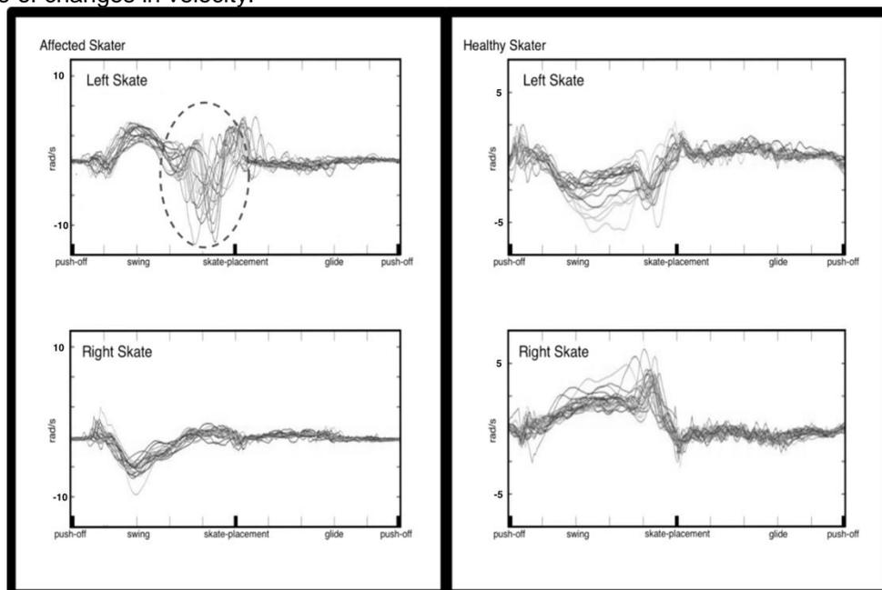
**Figure 3:** Participant two, looking at the results from another participant, we see a very different pattern of aberration, but the locality of the disorder and its regularity over multiple gait-cycles is apparent. This indicates the disorder is person-specific.
