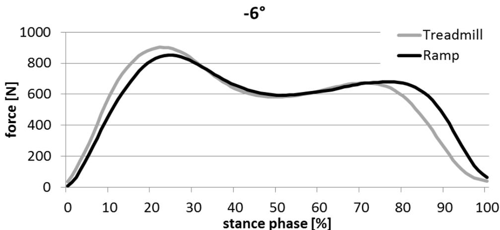
**Figure 1: Loadsol forces during stance phase in 6° downhill walking on a treadmill and ramp construction during stance phase.**
