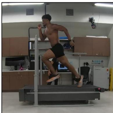
**Figure 1. Subject completing 5s run at 6.5 m/s on the instrumented treadmill.**
