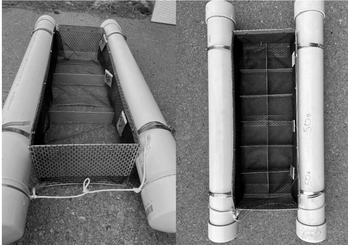
Figure 1. General design of a floating basket incubator (FBI). FBI 3-cell (left) and FBI 12-cell (right). Surface current supplies water to embryos resting in the floating basket which is supported by two pontoons constructed from PVC piping.
