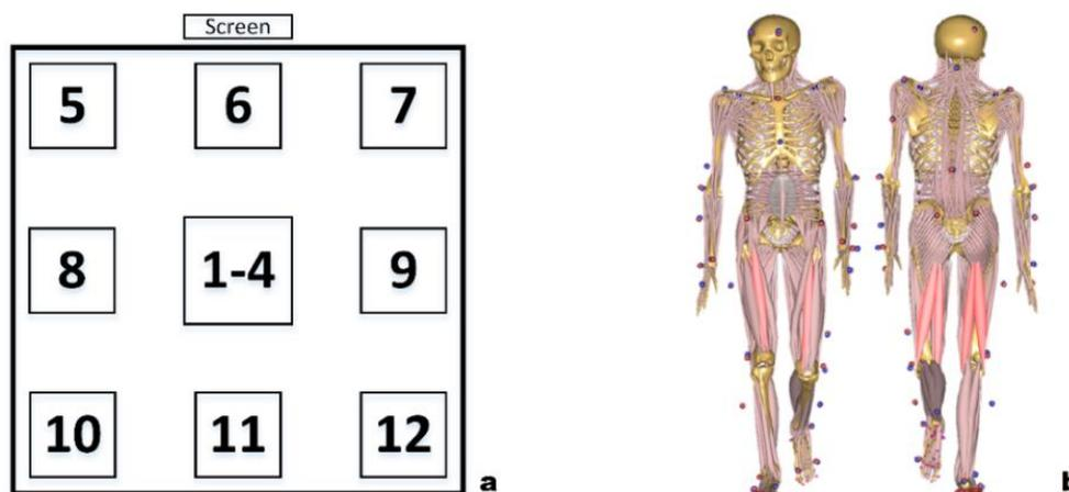
**Figure 1: a) Schematic view of the SpeedCourt system with the location and numeration of the pressure sensors. The sensors 1-4 in the middle were treated as one field for this study. b) Musculoskeletal model of the AnyBody Managed Model Repository (AMMR, v. 2.2.0).**
