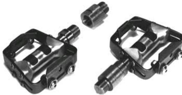
Figure 1: Diagram of Kneesavers™ device which was placed between pedal and crank arm. (Ice et al., 2008)
