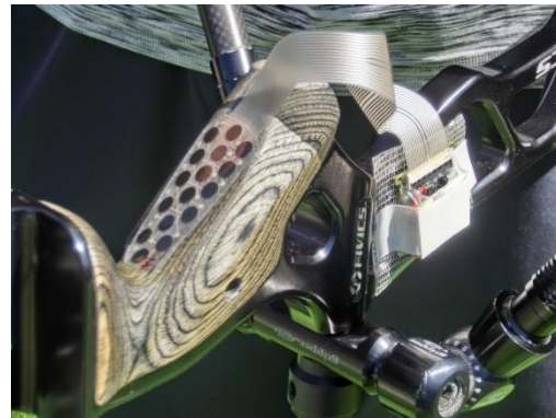
Figure 2: SETUP B - Experimental setup with IMU positioned on the riser, just below the grip.
