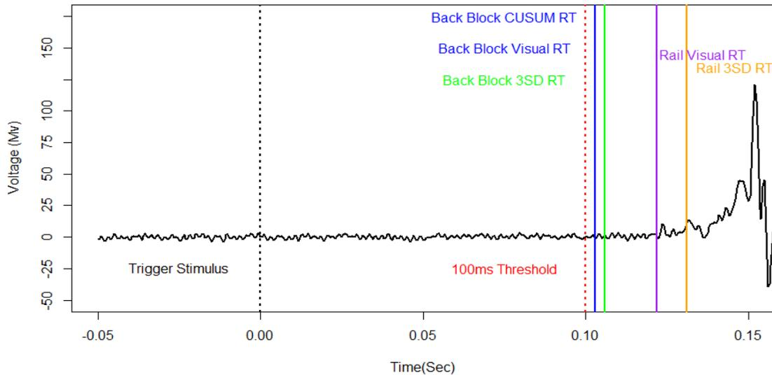
**Figure 1: Demonstrating rail accelerometer data and additional lines specifying the Trigger Stimulus (black), 100 ms Threshold (red), Back Block CUSUM RT and Back Block Visual RT (blue), Back Block 3SD RT (green), Rail Visual RT (purple) and Rail 3SD RT (orange), for a single trial.**
