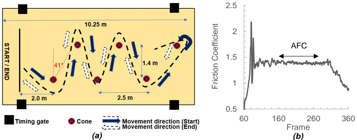
Figure 1: (a) Slalom course (b) Example of a typical friction coefficient curve
