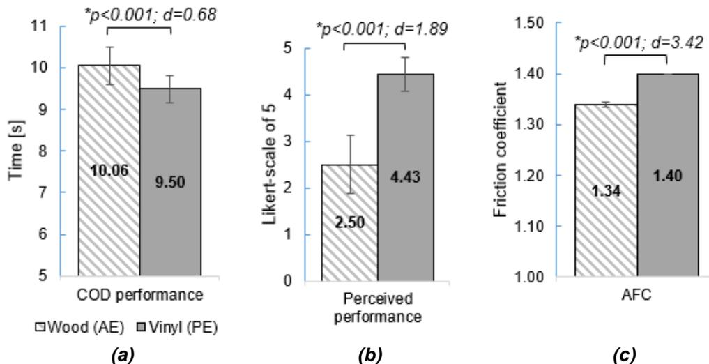
**Figure 2: Mean value ( $\pm$ SD) of (a) change of direction performance, (b) perceived traction performance and (c) available friction coefficient (\*t-test:  $p < 0.05$ ). Effect sizes are shown as Cohen's  $d$ .**
