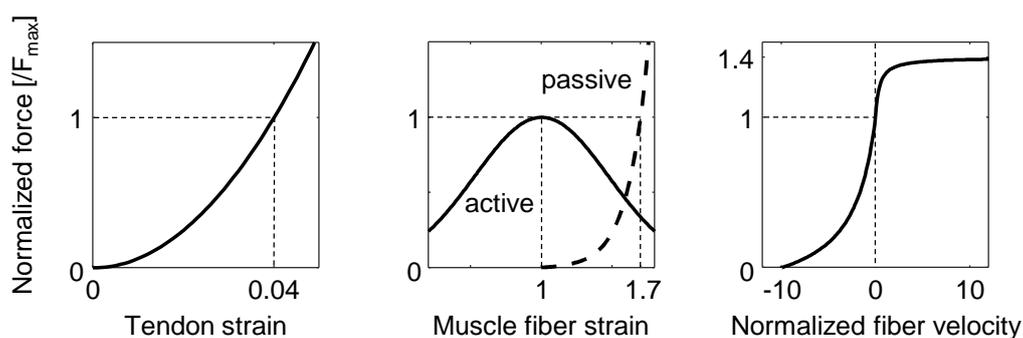
**Figure 1: Force-length-velocity relationships of the Hill-type musculotendon model.**
