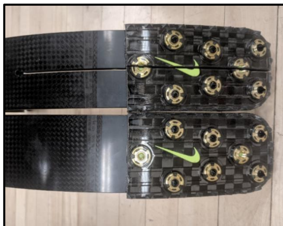
Figure 1. Split-toe (top) and solid (bottom) prostheses. Split-toe prosthesis differed only in the longitudinal cut on the distal end.
