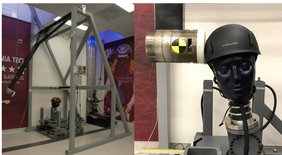
Figure 1: Photos of pendulum impactor (left) and side impact configuration with a representative rock climbing helmet model (right).
