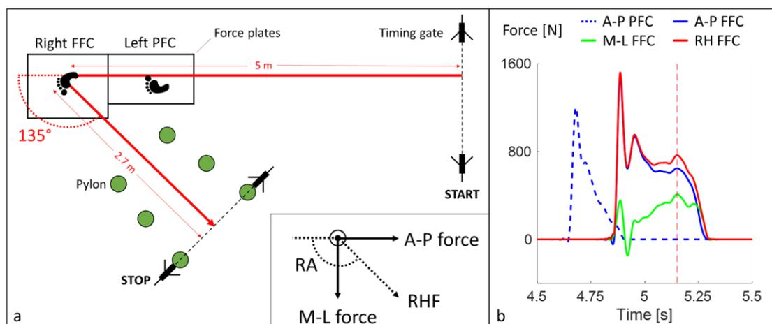
**Figure 1: 135-degree COD set-up (a). Example for ground reaction forces of one 135-degree COD (b). The dashed red line marks the peak horizontal propulsive force during push-off.**
