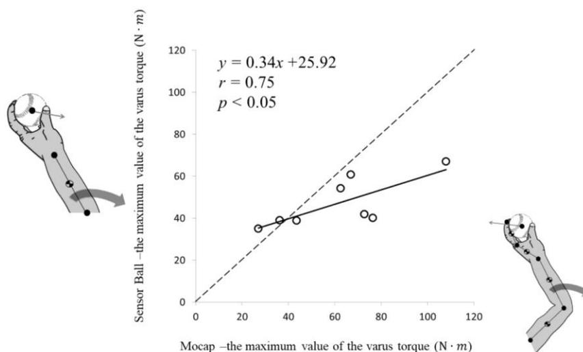
**Figure 2: The relationship between the maximum values of the varus torque calculated by the proposed method and the maximum values of the varus torque calculated by Mocap. A schematic drawing of the one and four segment was drawn for each.**
