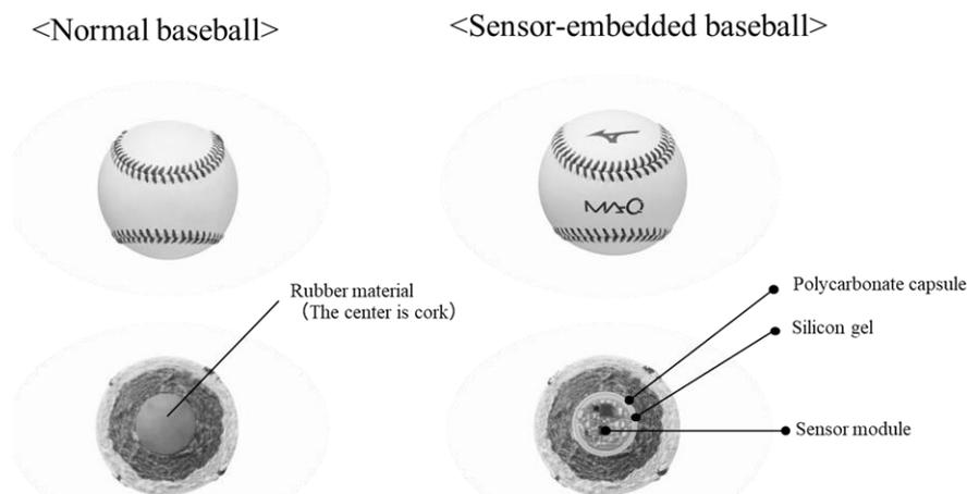
**Figure 1: Structure of a regular hardball and a sensor-embedded baseball.**
