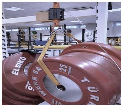
**Figure 1. 250-kg hanging from GSTRENGTH strain gauge with output USB connector.**
