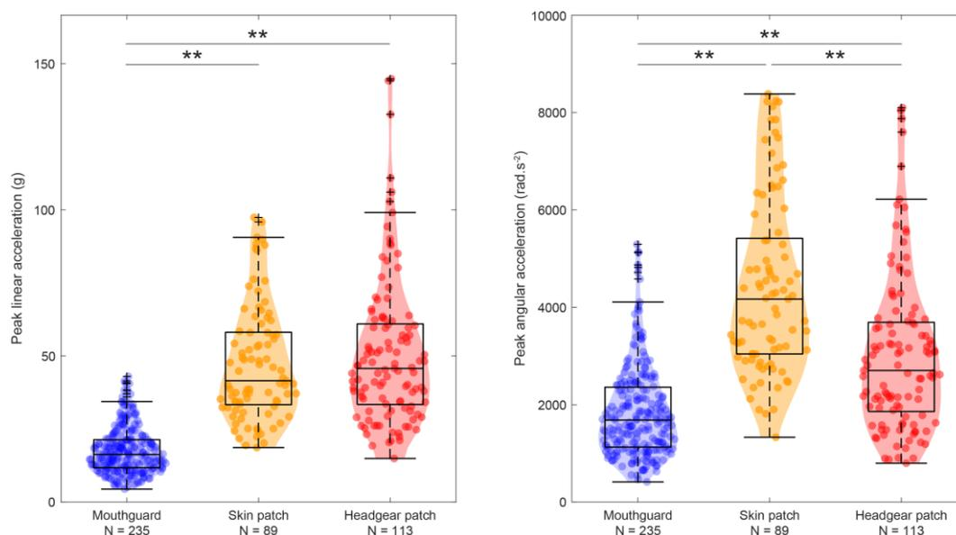
**Figure 2: Distribution of peak linear and angular accelerations for a subset of 'good' events representative of head motion. Asterisks indicate differences between sensors (\*\*p < 0.001).**
