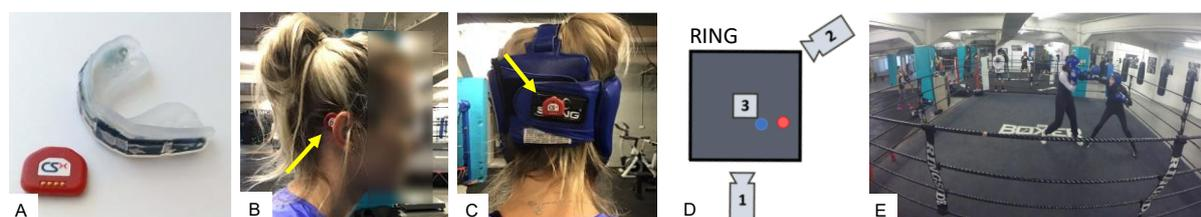
**Figure 1: (A) CSx patch and Prevent Biometrics Hybrid mouthguard; (B) location of the skin patch; (C) location of the headgear patch; (D) placement of cameras around the ring; (E) example of footage from camera 1.**
