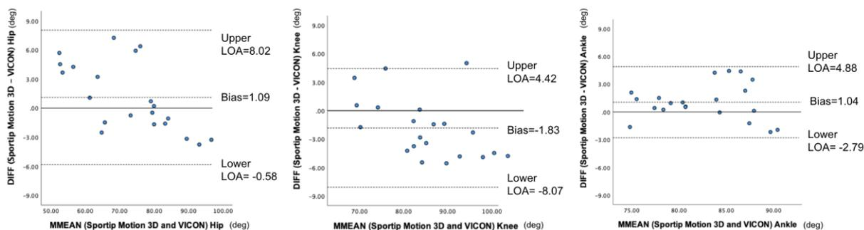
Figure 3: The Bland–Altman plot for each angle measured using Sportip Motion 3D and VICON.
