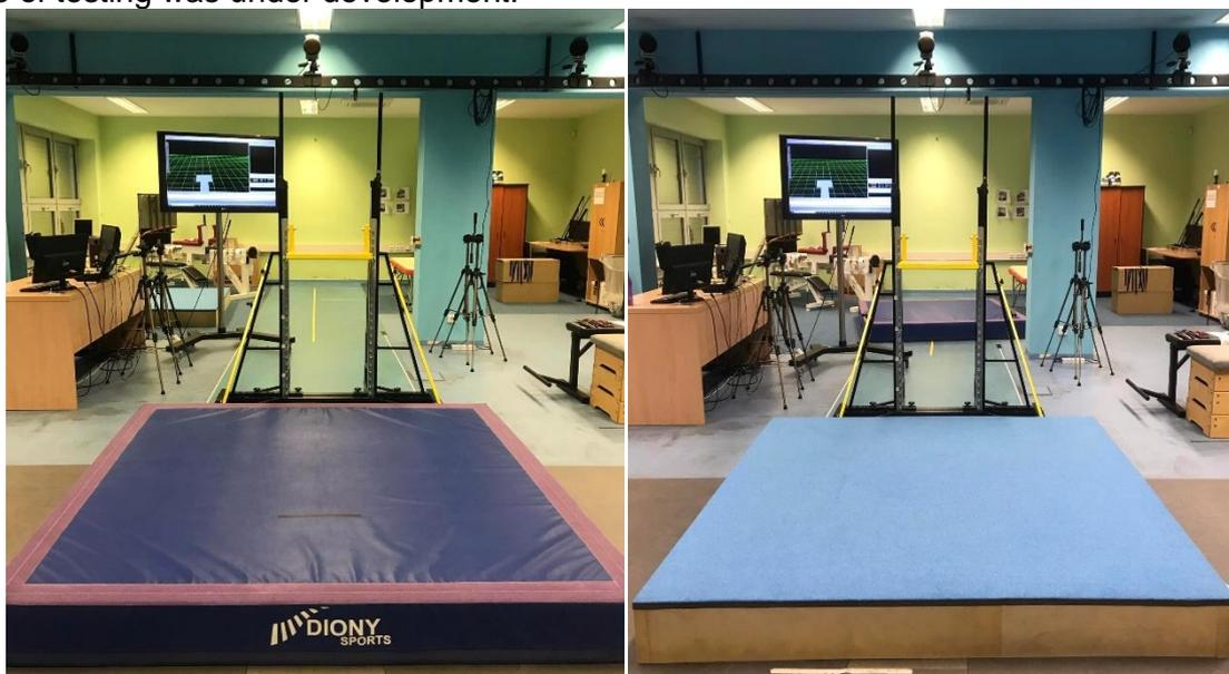
**Figure 1: Types of landing mats (right – REGULAR, left - PROTOTYPE)**
