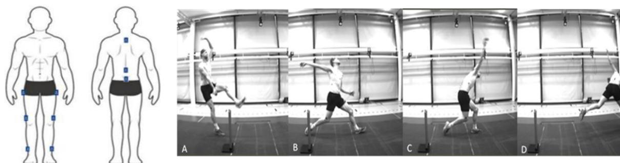
**Figure 1&2: Accelerometer locations (left) and Key instance identified (right) (A) BFC (B) FFC (C) Ball Release (D) FT.**
