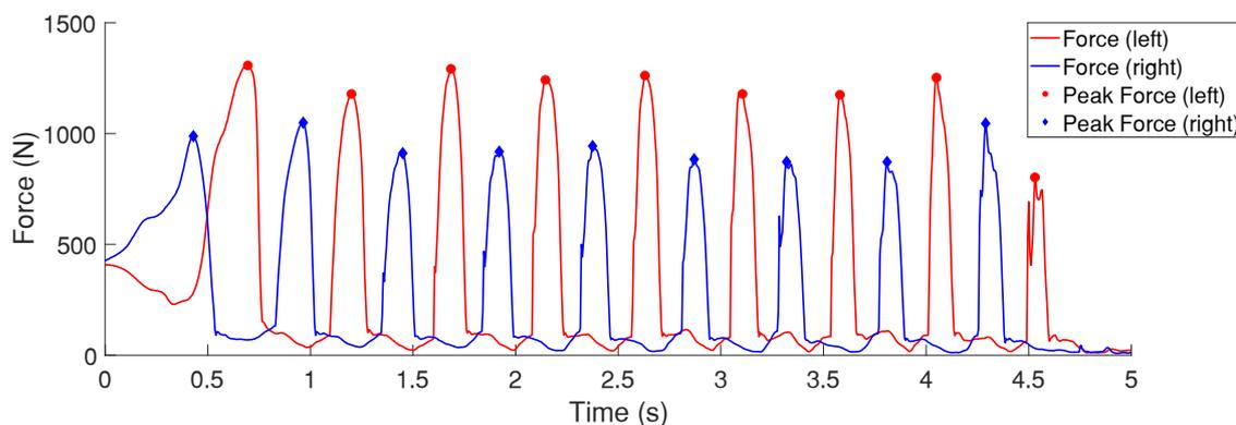
**Figure 1: Force vs time plot for one participant's push start trial with the left (outside) and right (inside) foot displayed in red and blue respectively. Peak force is indicated at each contact.**
