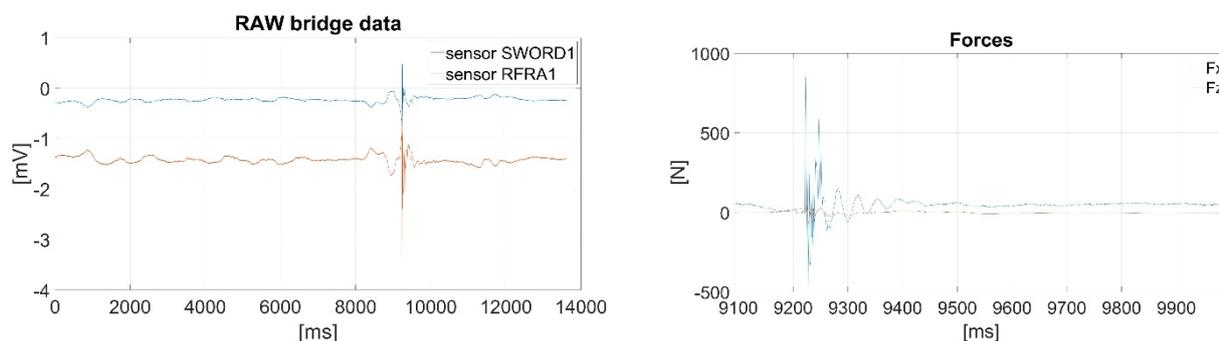
**Figure 3: example of data acquired during a controlled hit (left) and forces estimated for the impact section combining values of the two bridges using calibration parameters (right)**
