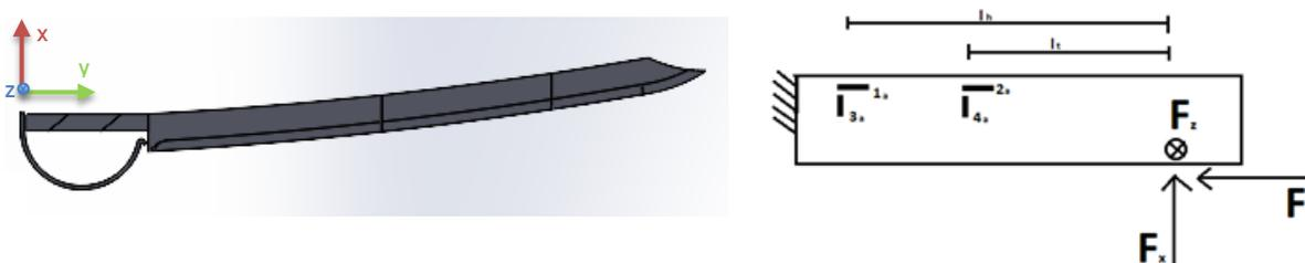
**Figure 1: FEM model of the sword with reference system (left) and scheme of the strain gauges arrangement on one side (right). Configuration was replicated also on the opposite face**
